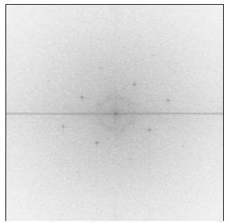
Figure 4: FFT Signature of Latent Print with High Frequency Halftone Background
